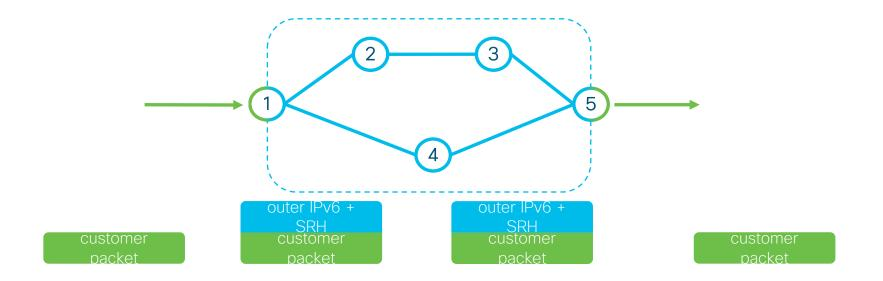
Egress PE removes the outer IPv6 header as the packet leaves the SR domain
